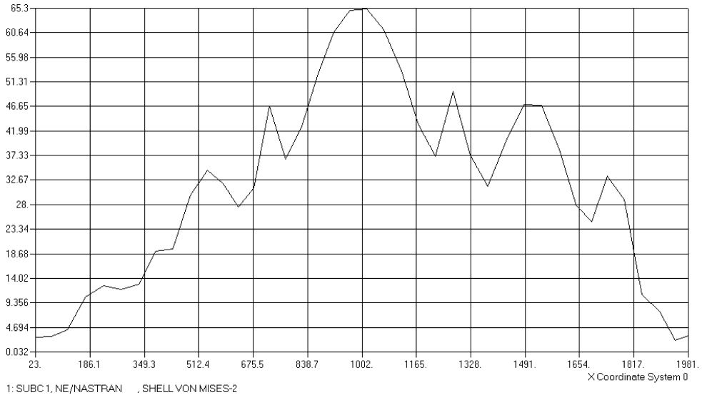
FIG. 11. Changes of the reduced stress values \sigma_H [MPa] along the mantle generating line. Original solution – total rope wound on the pulley [3].
