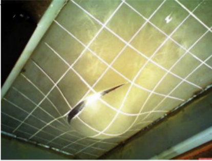
FIG. 11. Crack displacement in the grounding simulation: a) ALSOS and AMDAHL experiment [36], b) numerical simulation.
