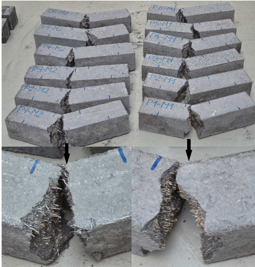
FIG. 10. Destroyed small-sized beams P1-M1 ÷ P6-M1 and P1-M2 ÷ P6-M2.
