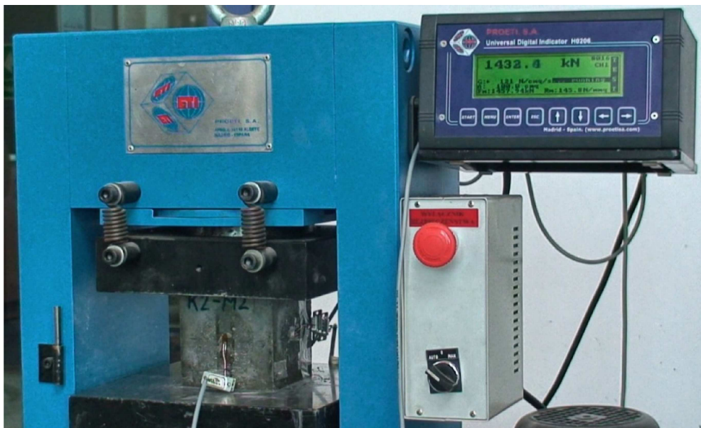
FIG. 6. The test stand for testing cubes K1-M1 ÷ K6-M1 and K1-M2 ÷ K6-M2.
