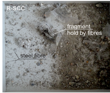
FIG. 14. View of the specimen after the test with a strain rate of 193 \text{ s}^{-1} .
