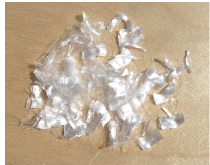
FIG. 1. View of a) recycled steel fibres and b) polypropylene fibres.
